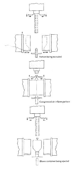
Extrusion blow molding
